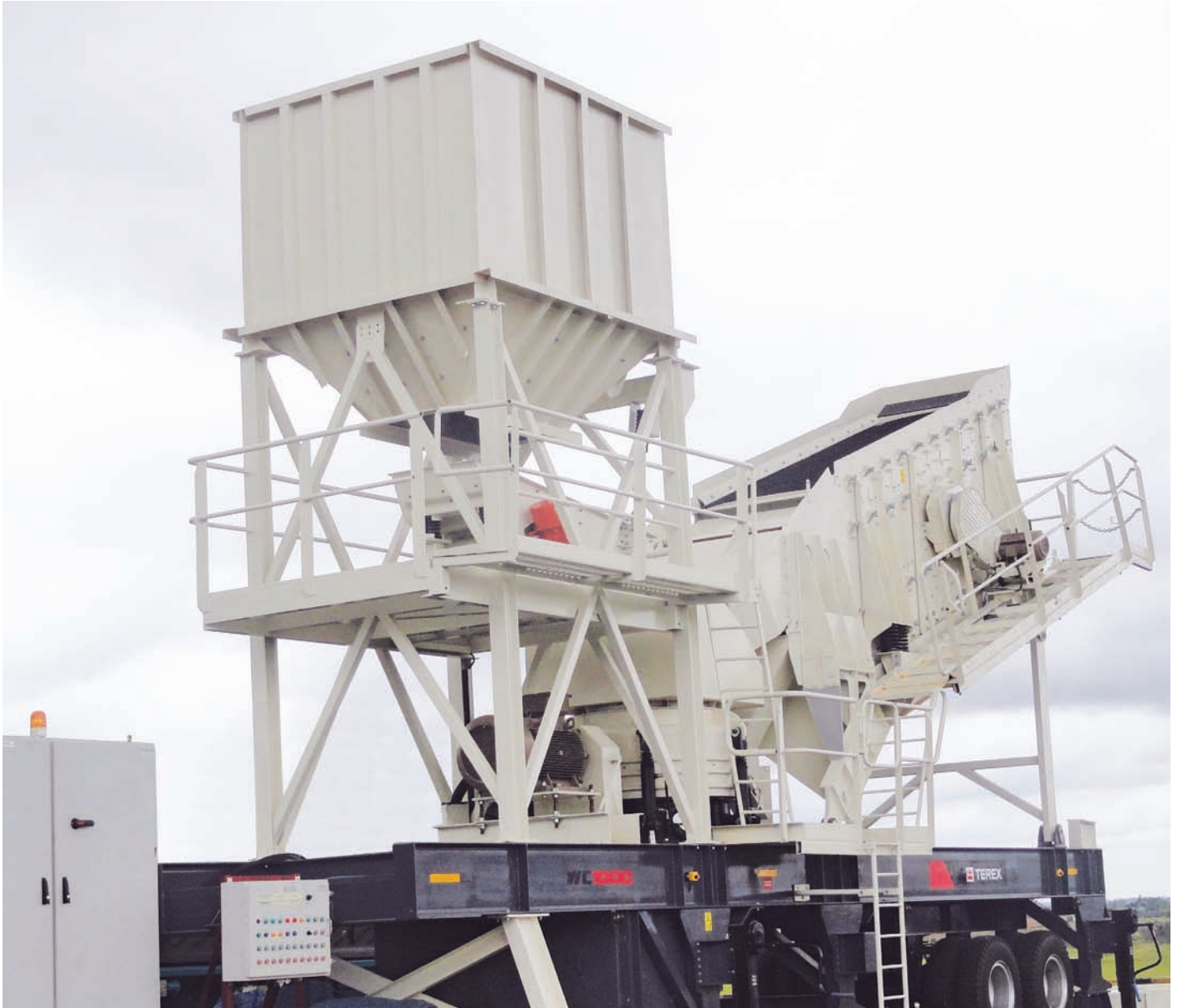
WC1000 Wheeled Cone Plant shown in operating mode with the surge hopper and pan feeder mounted on the chassis.
